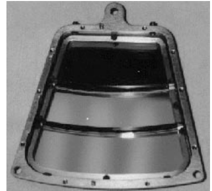
Fig. 15: A picture of three ‘‘ramp filters’’ in a filter cell that mounts into the filter wheel.
